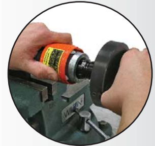
Quick Change Tooling: PTO Coupling allow for quick tool changes.
